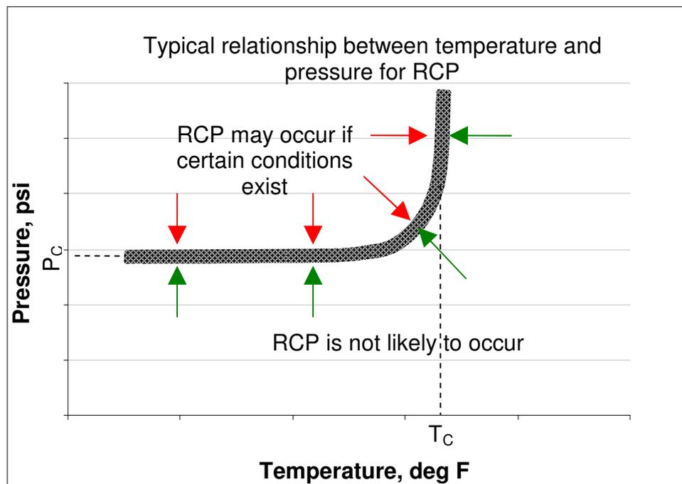
**Figure 1: Critical Temperature,  $T_C$  and Critical Pressure,  $P_C$**
