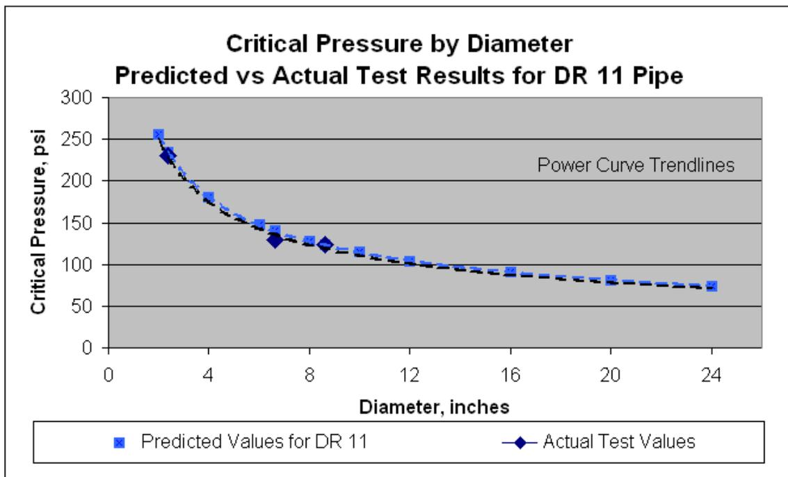
**Figure 3: Critical Pressure by Diameter – Predicted versus Actual Test Values**
