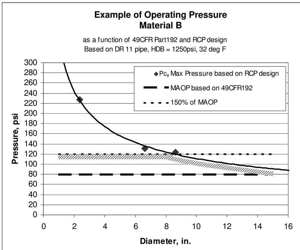
**Figure 4: Operating Pressure as a Function of Diameter and Full scale Critical Pressure,  $P_c$**
