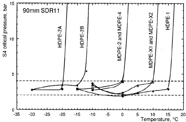
**Figure 2: RCP Characteristics of Various PE Pipe Grades (10)**
